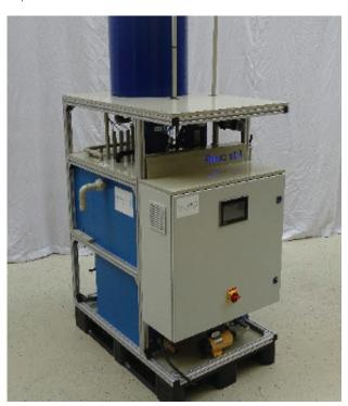
A small MD pilot with a full size module and a total membrane area of 26m² was integrated within a waste water stream inside a dye producing factory. Cooling water was taken from a pond and heat was electrically generated because of scale.
