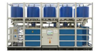
Middle size production system for water treatment from saline water streams.
