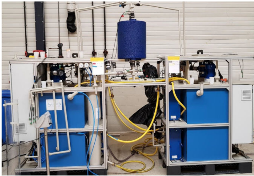
Fig. 7. Actual setup used in this work. Module can be seen in the middle, with the valves on top and at the bottom of the outlet and inlet. On the left and the right, the two individual pilots can be seen.
